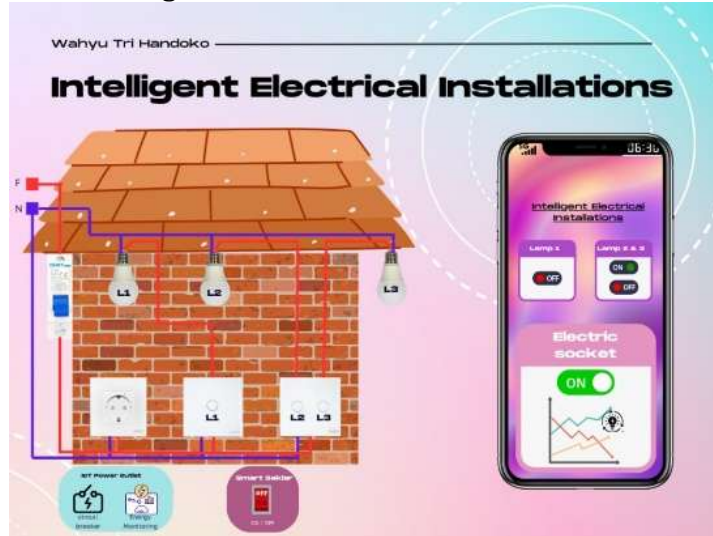
Figure 2. Intelligent Electrical Installation Kit Trainer Design
