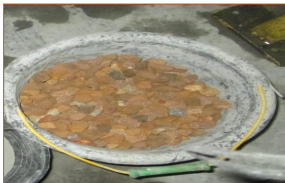
Figure 1. Physical appearance of Sei Sembuluh river sand used as fine aggregate
