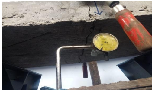
Figure 7 Reading of the Dial Gauge at the moment Plate in Crisis Cracked Conditions
