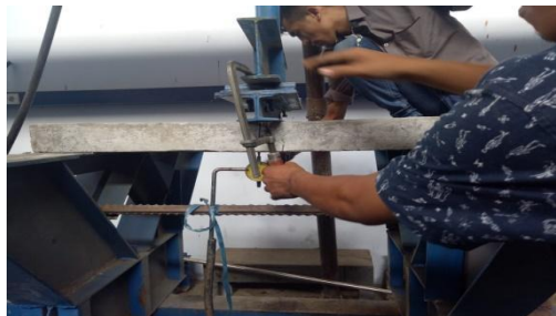
Figure 5 Preparation of the Plate Bending Strength Testing Process
