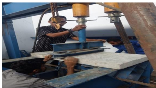
Figure 6 View of the Placement of the Plate on the Test Tool
