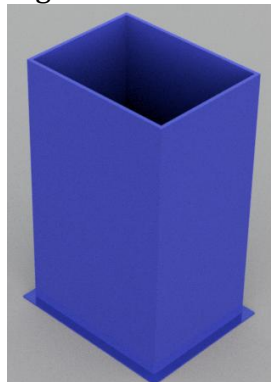
Figure 1. 3D Model of Hollow Crash Box Used as Baseline Control to Compare Structural Response Against Lattice-Based Configurations
