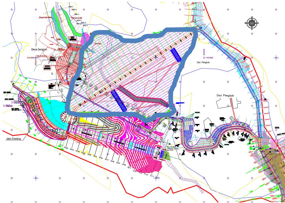
Figure 2. Layout Plan of the Main Dam Embankment
