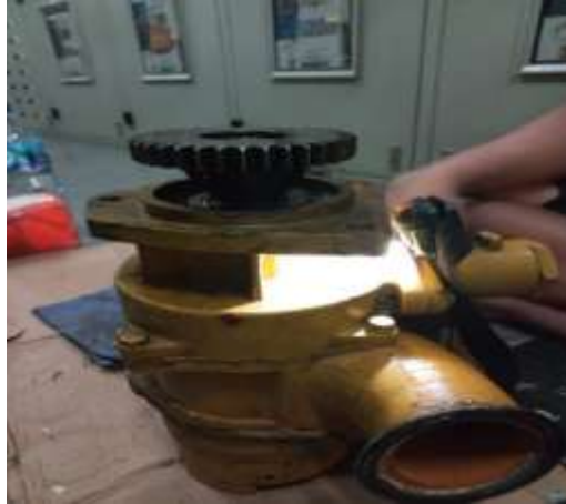
Figure 5 Patched Seawater Cooling Pump Cover
