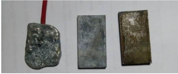
Figure 23. Specimen corrosion results for 432 hours.
