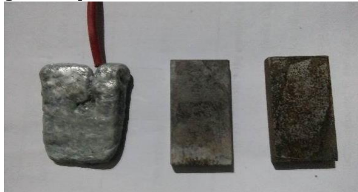
Figure 24. Specimen corrosion results for 576 hours.
