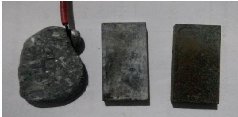
Figure 25. Corrosion results for 720 hours.
