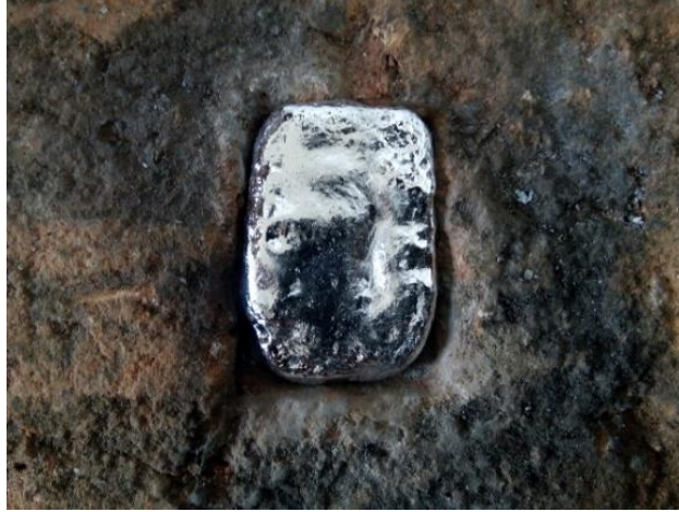
Figure 8. Anode Zinc (Zn) 99,99%
